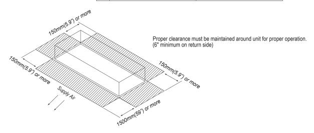
Samsung WindFree  $^{\text{TM}}$  1-Way Cassette, Single Zone, Split System AC009BXADCH/AA Dimensional Drawing
