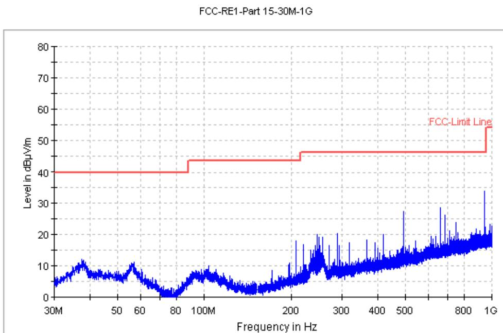
Fig.21. Radiated emission: GFSK, 2440MHz, 30 MHz - 1 GHz
