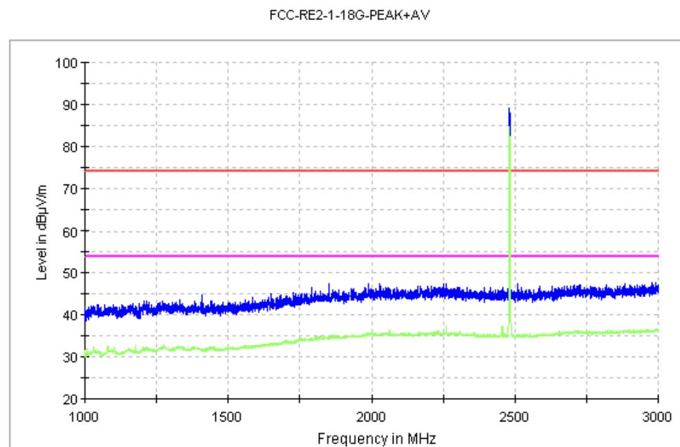
Fig.18. Radiated emission: GFSK, 2402MHz, 1 GHz - 3GHz
