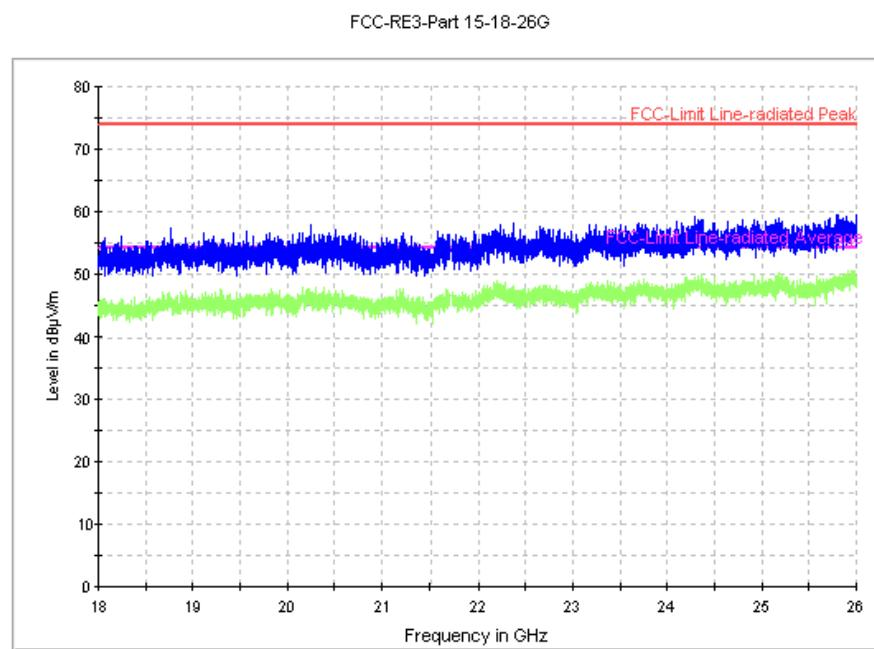
Fig.28. Radiated emission: GFSK, 18 GHz - 26 GHz
