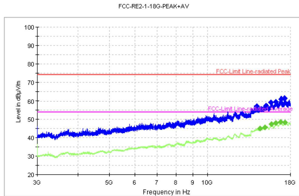
Fig.25. Radiated emission: GFSK, 2480MHz, 3 GHz - 18 GHz
