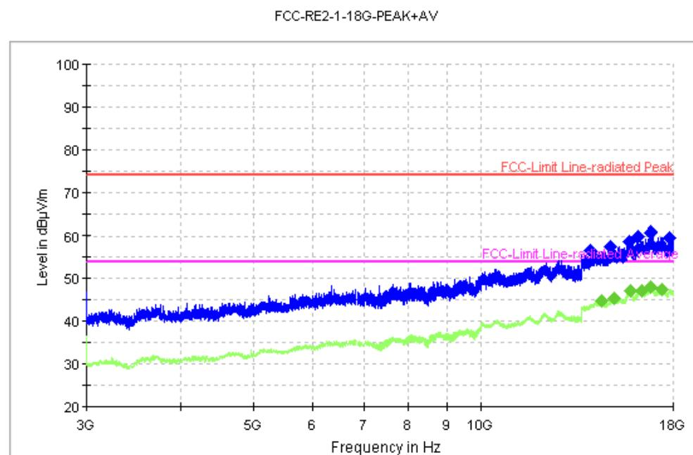
Fig.19. Radiated emission: GFSK, 2402MHz, 3 GHz - 18 GHz
