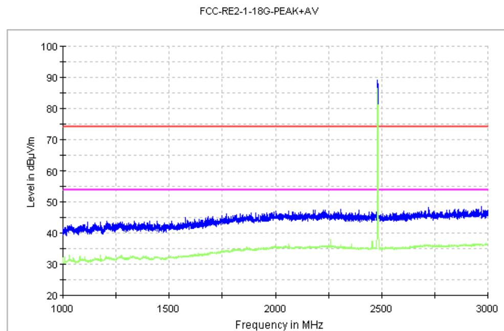
Fig.24. Radiated emission: GFSK, 2480MHz, 1 GHz - 3 GHz
