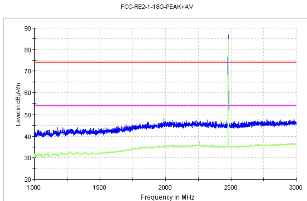
Fig.22. Radiated emission: GFSK, 2440MHz, 1 GHz - 3 GHz
