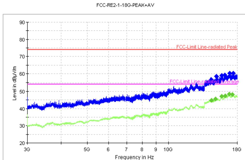
Fig.23. Radiated emission: GFSK, 2440MHz, 3 GHz - 18 GHz
