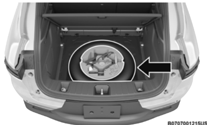
Damaged Tire Stowage
