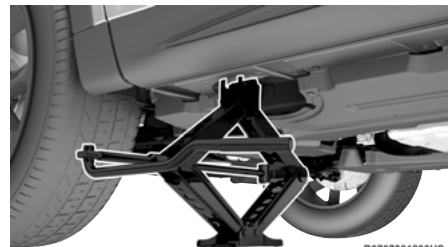
Front Jacking Location
