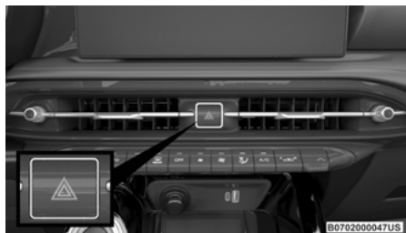
Hazard Warning Flashers Button
