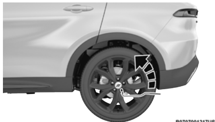
Loosening The Wheel Bolts
