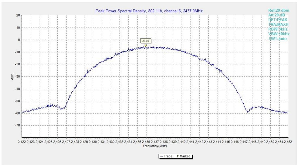
Fig.B.3.2 Power Spectral Density (802.11b, Ch 6)
