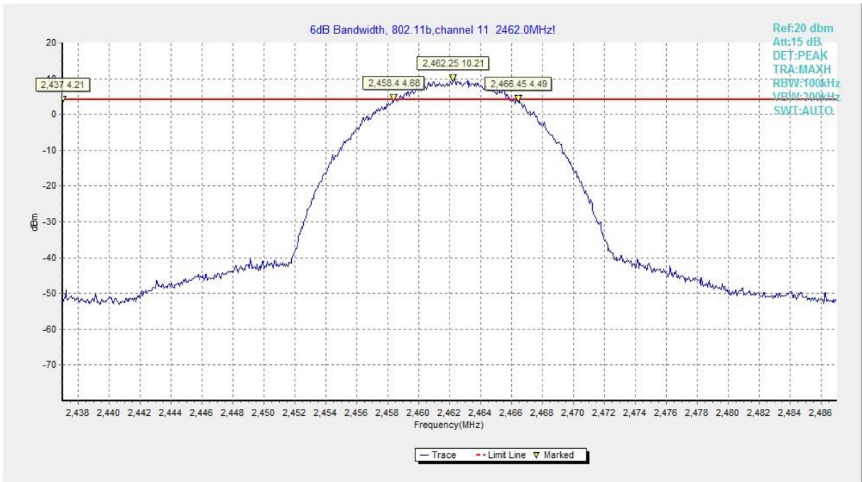
Fig.B.4.3 Occupied 6dB Bandwidth (802.11b, Ch 11)
