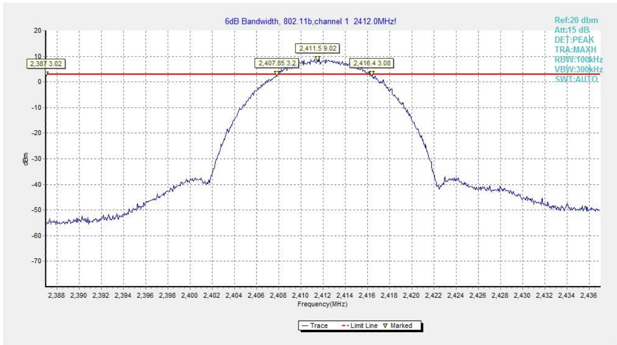
Fig.B.4.1 Occupied 6dB Bandwidth(802.11b,Ch 1)
