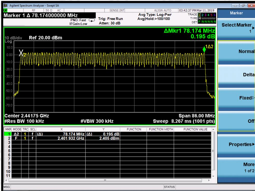
Note: All modes were tested, the test records reported is modulation GFSK.
