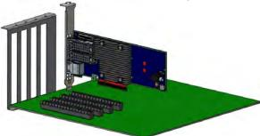
3. Applying even pressure at both corners of the card, insert the DPU into the PCI Express slot until firmly seated.
