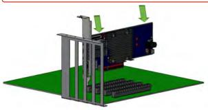
4. When the DPU is properly seated, the port connectors are aligned with the slot opening, and the DPU faceplate is visible against the system chassis.
