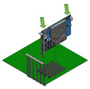
4. When the DPU is properly seated, the port connectors are aligned with the slot opening, and the DPU faceplate is visible against the system chassis.
