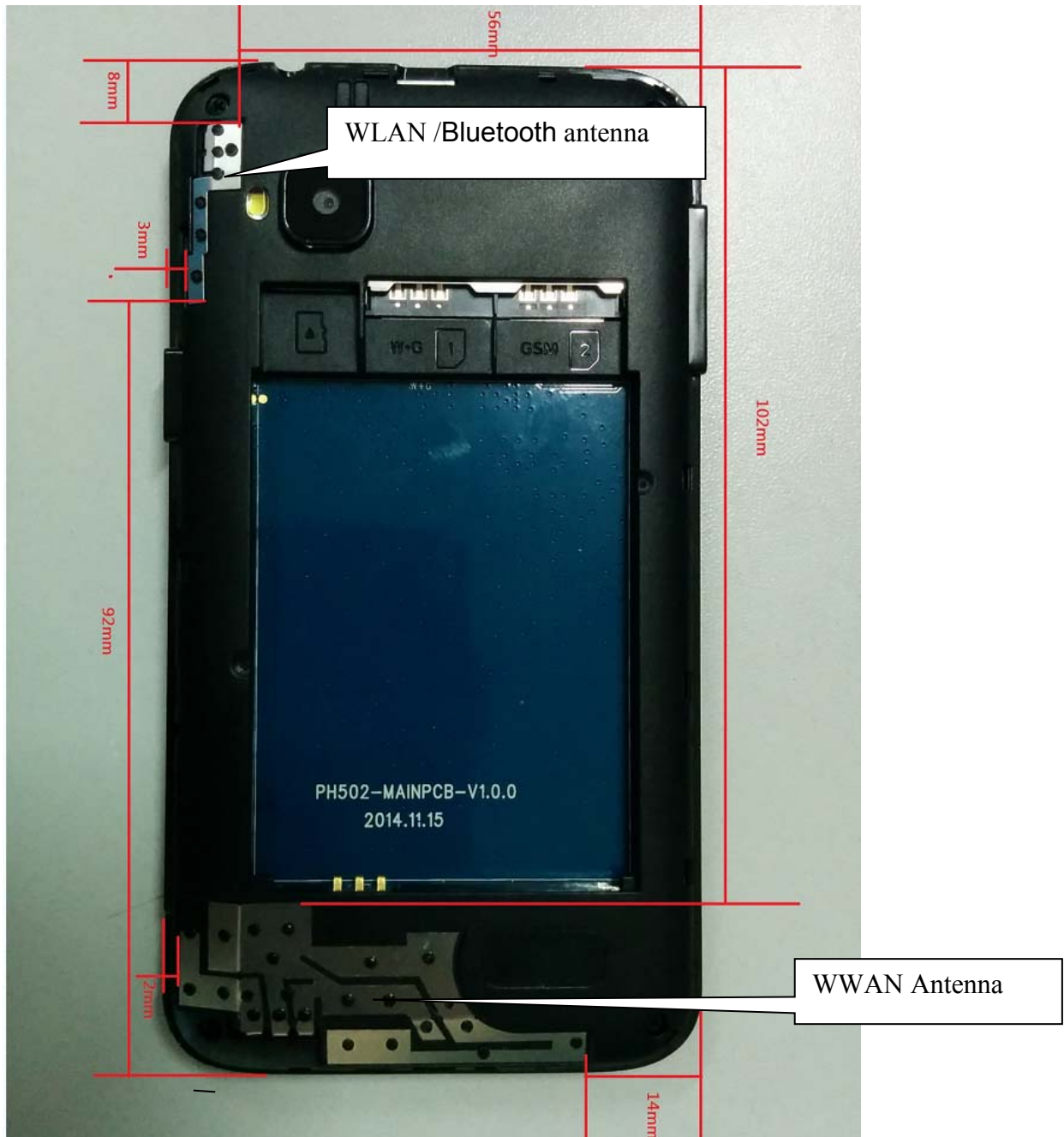
Mobile Hotspot Sides for SAR Testing
