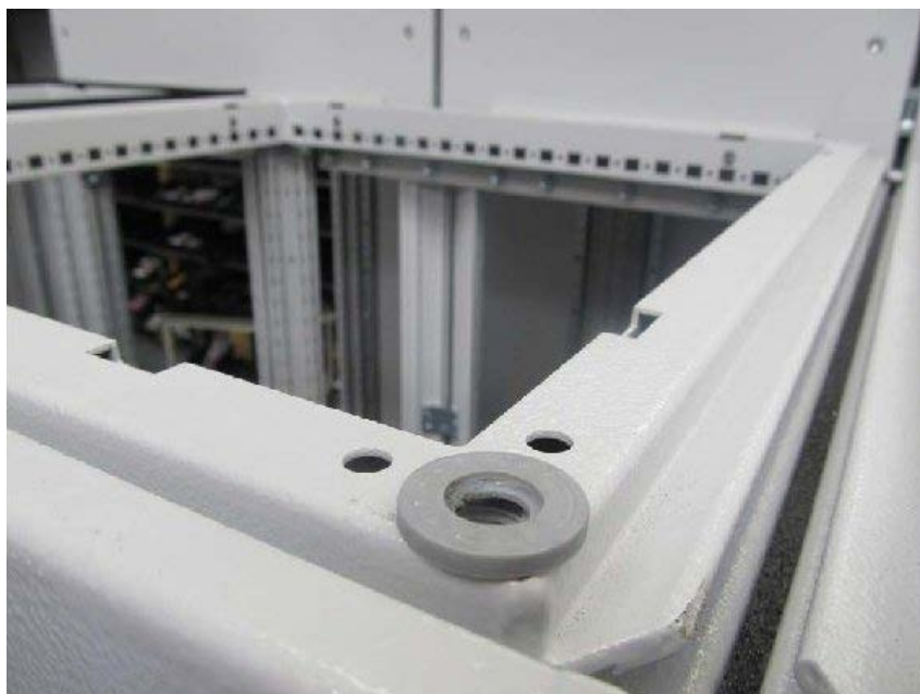
Figure 3-18 Attaching the washers
