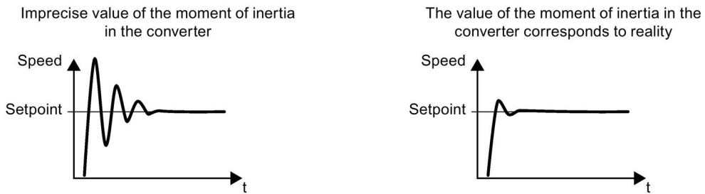
Figure 9-28 Influence of the moment of inertia estimator on the speed
