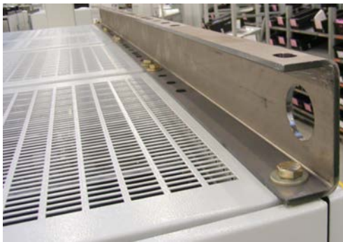
Figure 3-8 Option M90, transport beams
