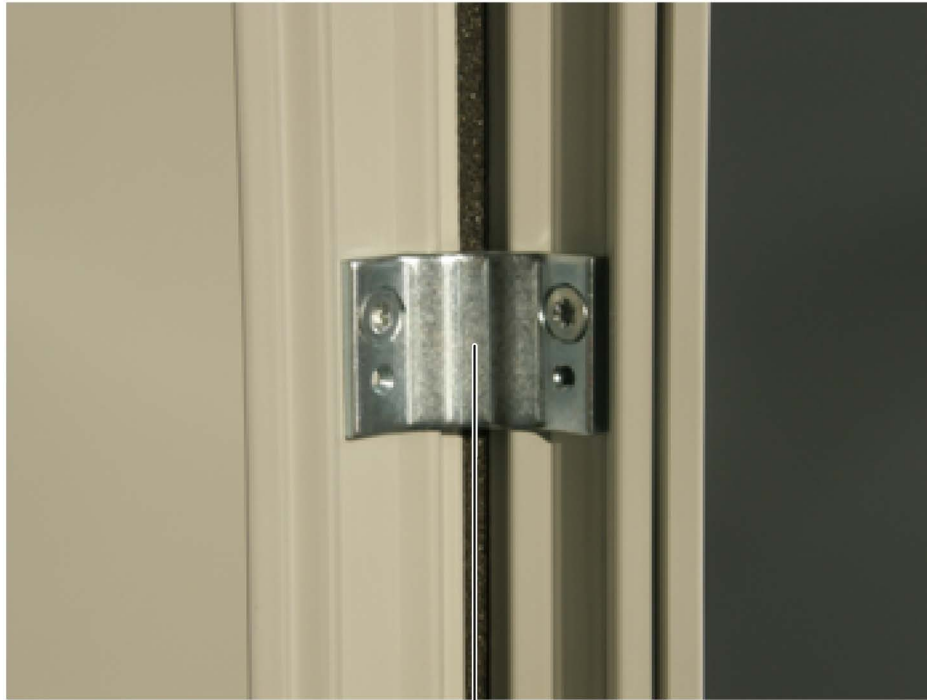
Outer cabinet connector Tightening torque: 9 Nm
