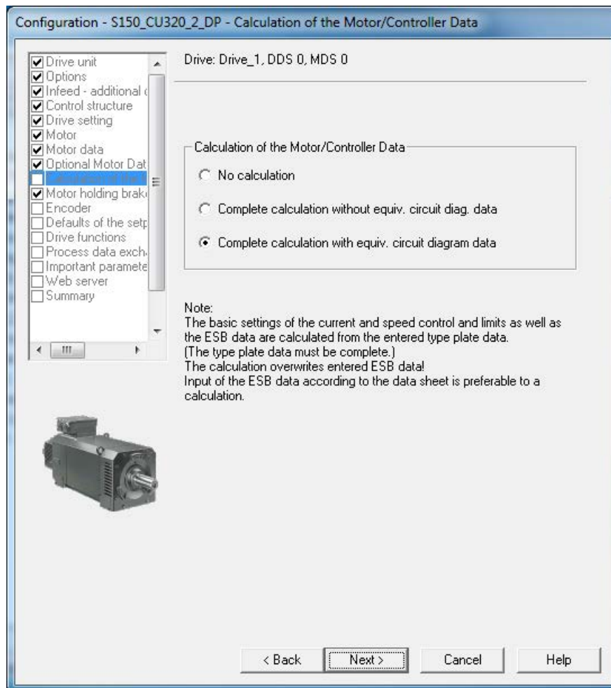
Figure 5-24 Calculating the motor/controller data
