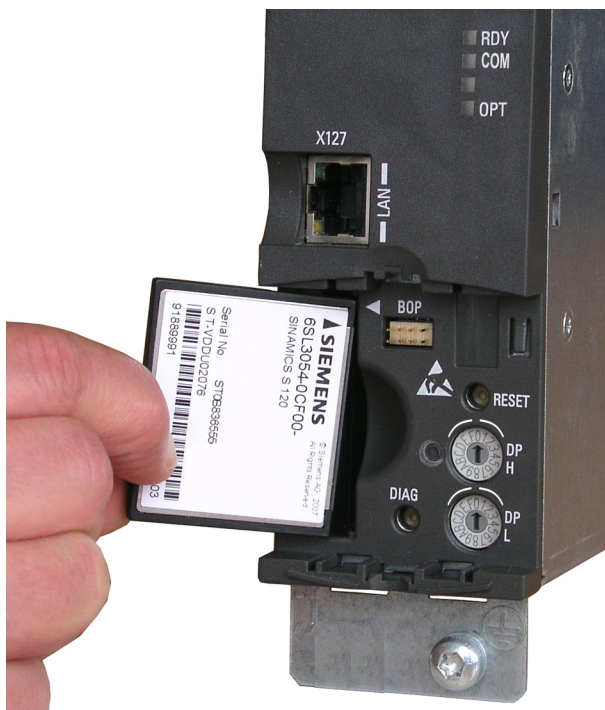
Figure 4-15 Slot for the memory card
