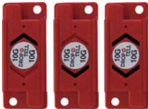
Figure 3-5 Shock indicator tripped
