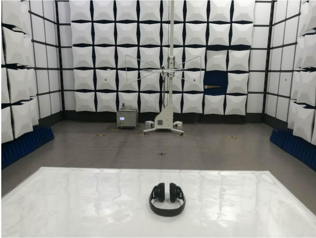
FCC RADIATED EMISSION TEST SETUP
