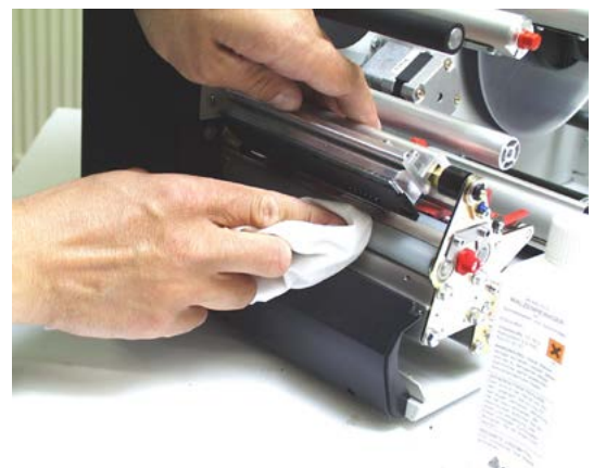
Fig. 4 Rotate the printhead upwards before cleaning it.
