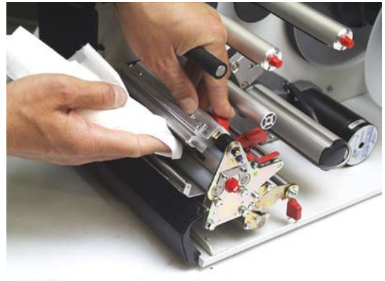
Fig. 1 Cleaning of the printhead – the printhead needs not to be unplugged (Fig: Dispenser version).
