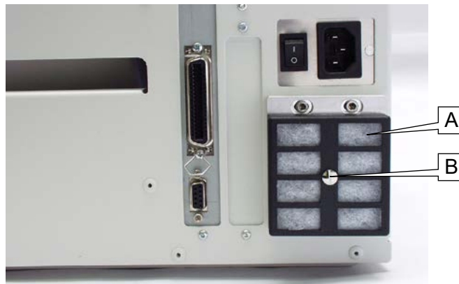
Fig. 7 64-08 with mounted dust filter (A).
