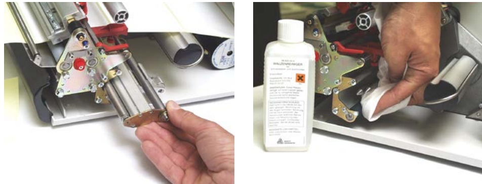
Fig. 6 Left side: pulling out the pull-out module; right side: cleaning the dispenser-feed-roller using roller cleaner.
