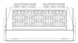
Accessory Air Filter Box for 1" or 2" Air Filters. Filter Size Adjustment knob is on both sides.
