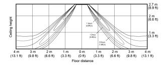
Cooling temperature distribution (Discharge angle: 45 degree)
