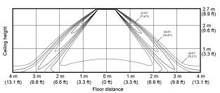
Heating temperature distribution (Discharge angle: 52 degree)
