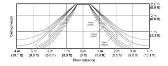
Cooling temperature distribution (Discharge angle: 45 degree)
