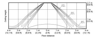
Heating temperature distribution (Discharge angle: 52 degree)
