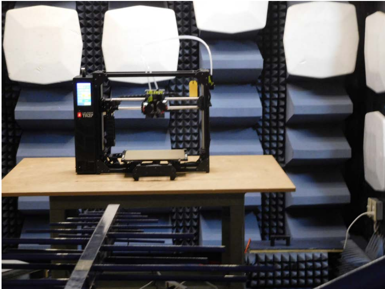
Test setup for Radiated Emissions
