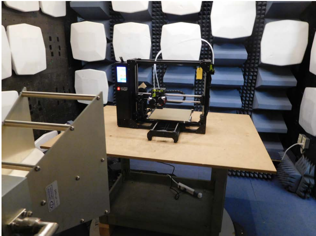
Test setup for Radiated Emissions
