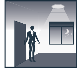
With insufficient ambient light, the sensor switches on the lamp when motion is detected
