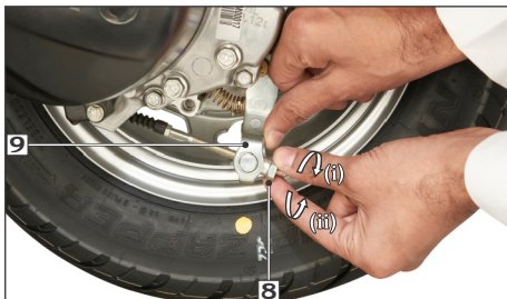
(8) Adjuster nut (9) Brake arm (i) Decrease free play (ii) Increase free play
