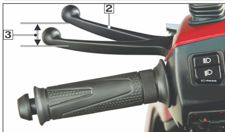
(2) Integrated brake lever (3) Free play 10-20 mm
