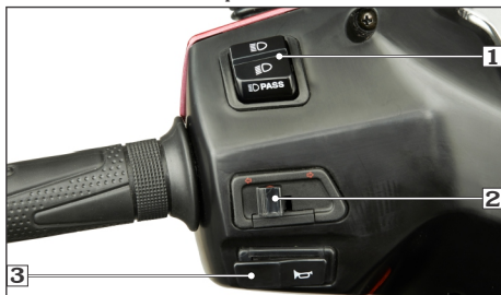
(1) Dimmer switch/Passing switch (For VX model only) (2) Turn signal switch (3) Horn switch
