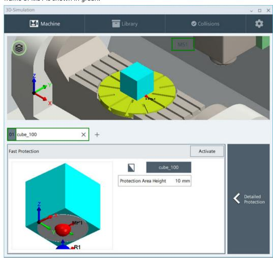
Figure 6-49 Active setup with "Fast Protection" The mounting point (red) lies centered at the lower side of the blank.
