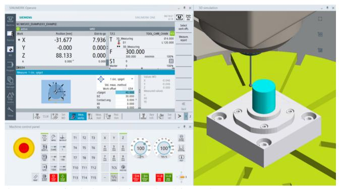
Figure 6-57 Measuring using the example of a measuring cycle in JOG mode
