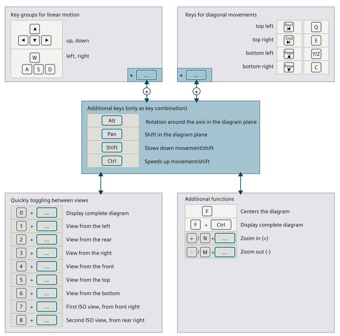
Figure 6-6 Functions of keys in 3D simulation
