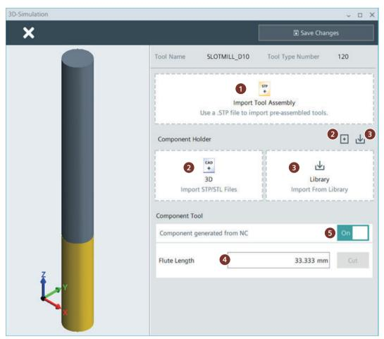
Figure 6-29 Overview of detailed protection for a tool defined using the example of an end mill
