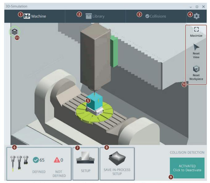
Figure 6-1 3D simulation, operating areas and functions using the example of a milling machine
