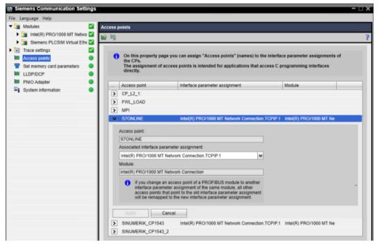
Figure 4-2 Setting the access point
