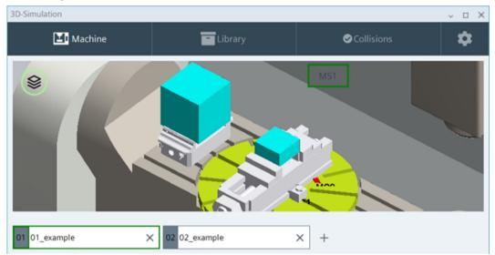
Figure 6-53 Example, milling machine with one mount station (MS1): Two setups are defined and activated
