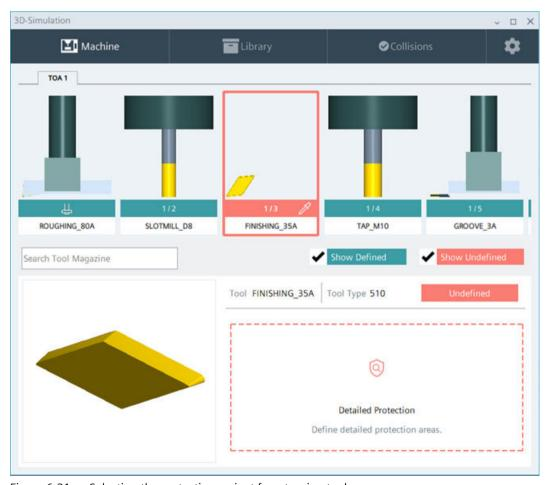
Figure 6-31 Selecting the protection variant for a turning tool
