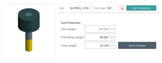
Figure 6-28 Fast protection for a tool defined using the example of an end mill
