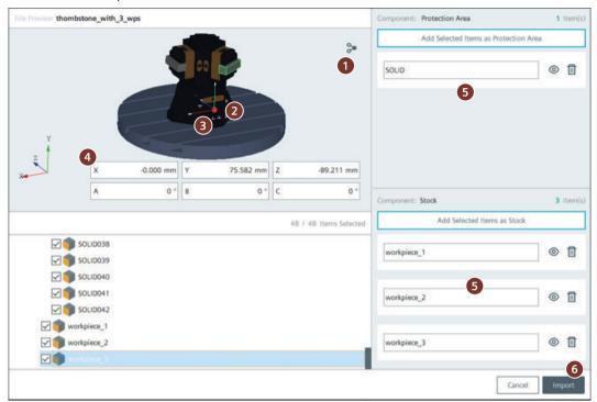
Figure 6-23 Setting the mounting point in the 3D model
