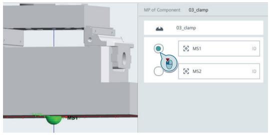
Figure 6-21 The mounting point of the blank is assigned mount station MS1
