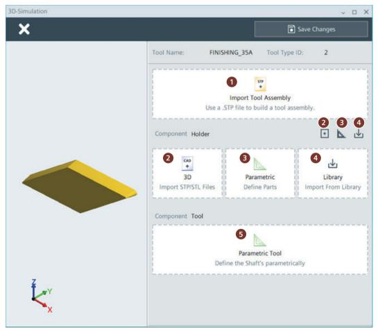
Figure 6-32 Detailed protection: Defining detailed protection for a turning tool
