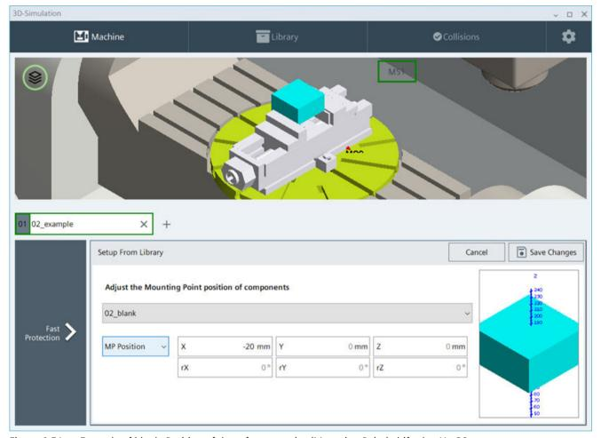
Figure 6-51 Example of blank: Position of the reference point (Mounting Point) shifted to X=-20 mm
