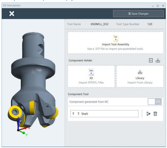
Figure 6-45 Importing the tool geometry as "\*.stp" file (shank and indexable inserts)
