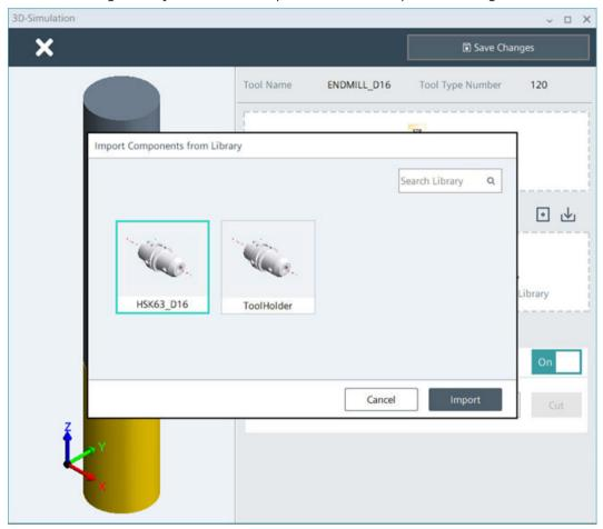
Figure 6-41 Importing a tool holder geometry from the library
