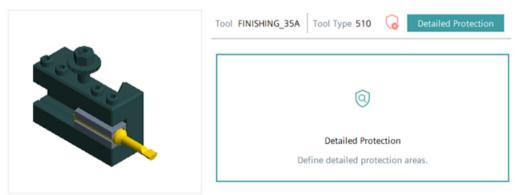
Figure 6-38 Detailed protection: Example of an end mill with imported geometries of the tool holder and the tool
