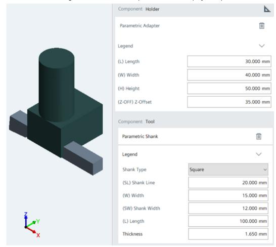
Figure 6-44 Defining a parametric adapter using a turning tool as an example
