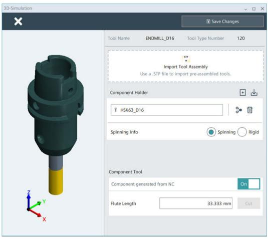
Figure 6-42 Tool holder from the library assigned to the tool
