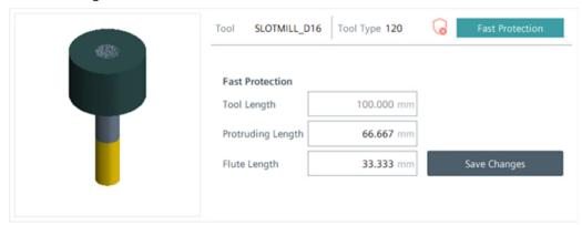
Figure 6-34 Defining fast protection for tool using the example of an end mill
