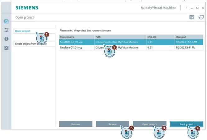
Figure 5-5 Opening a project in Run MyVirtual Machine
