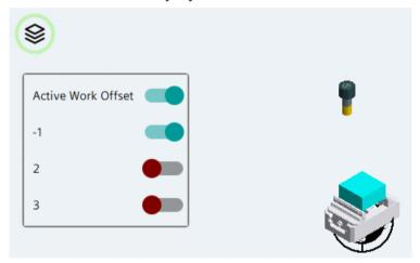
Figure 6-7 Showing and hiding a layer: machine housing and table hidden
