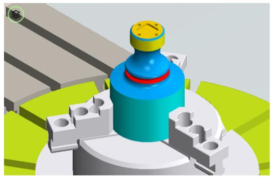
Figure 6-47 Stock removal simulation Machined surfaces are displayed in the colors of the tool cutting edges
