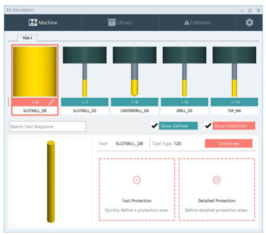
Figure 6-27 Selecting the protection variant for a tool
