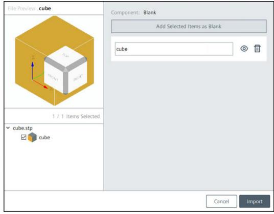
Figure 6-14 Example, blank with a component imported as "\*.stp" file
