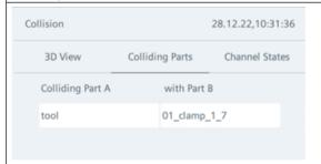
Which components are involved in the collision, e.g. tool, protection area, machine component
