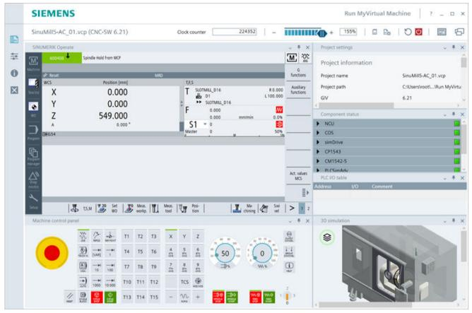
Figure 5-4 Run MyVirtual Machine: machine project newly created from the template after running up
