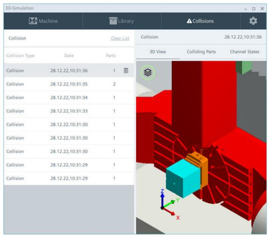
Figure 6-56 Collision screenshot, components involved are shown in color
