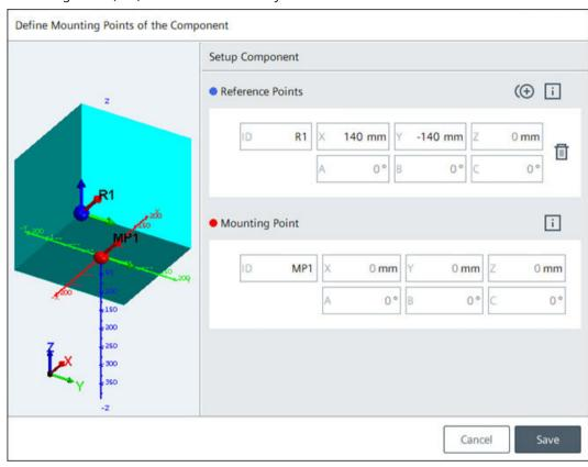
Figure 6-15 Example of blank: Reference point left-hand corner, Mounting Point, centered at the lower side.
