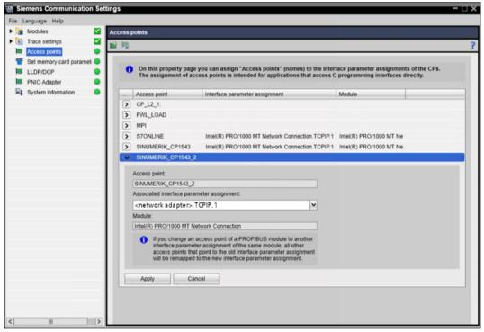
Figure 4-4 Setting the second access point CP1543\_2
