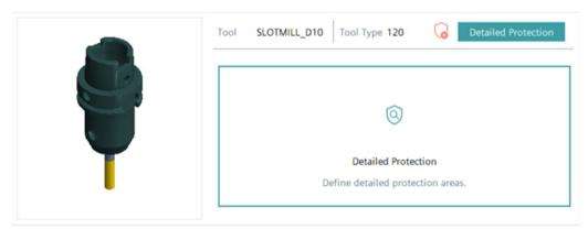
Figure 6-30 Detailed protection for a tool defined using the example of an end mill with a holder from the library
