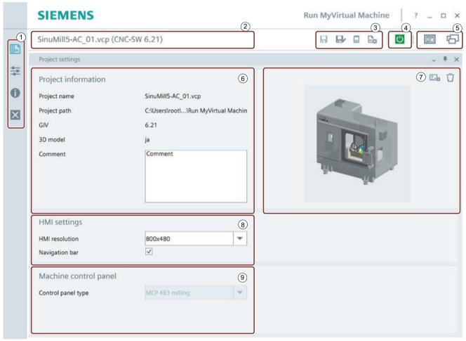
Figure 4-1 Project settings using a milling machine as example
