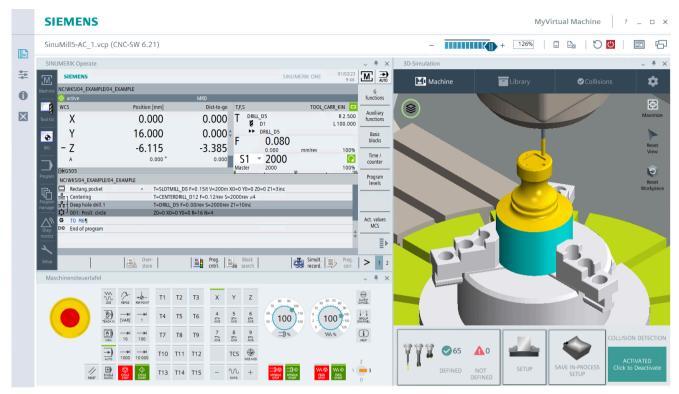
Figure 6-58 Example: simulation of machining process
