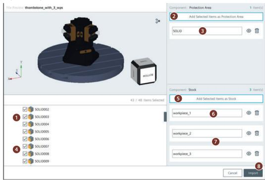
Figure 6-22 Importing a clamping tower with blanks as new setup
