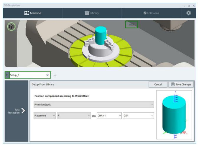
Figure 6-52 Reference point R1 of the blank is connected with work offset G54
