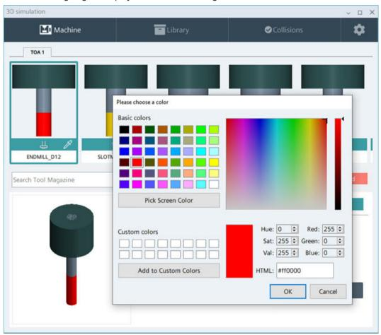
Figure 6-46 Example of an end mill: Defining a cutting edge color for a tool
