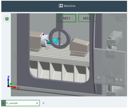
Figure 6-55 Example, mount station MS1 is active and configured
