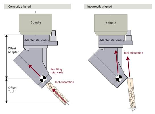
Figure 6-26 Angle head at 45° with specification of the relevant key variables
