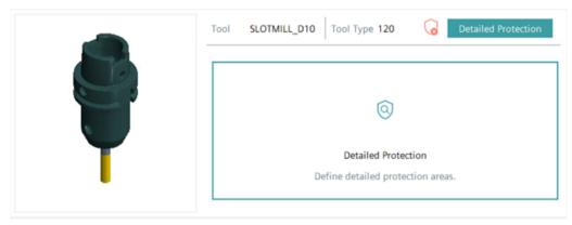
Figure 6-37 Detailed protection: Example of an end mill with imported tool holder geometry
