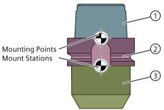
Figure 6-35 Example of tool holder, comprising three part geometries
