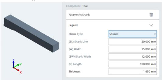
Figure 6-43 Defining the turning tool shank using parameters using a square shank as example
