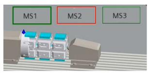
Figure 6-54 Examples of mount stations: MS1 configured and active, MS2 not configured, MS3 configured and not active
