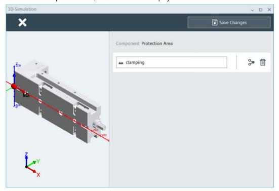
Figure 6-19 Protection area created from a STEP model
