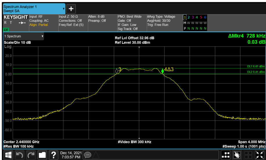
Figure 224 - Core 2 (C) 2440 MHz (CH17) 6 dB Bandwidth
