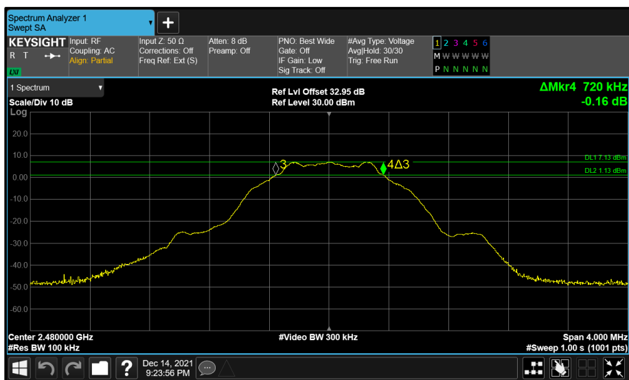
Figure 242 - Core 0 (A) 2480 MHz (CH39) 6 dB Bandwidth
