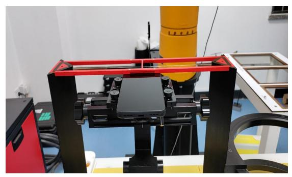
Picture 2: EUT Positioning for RF/T-coil
