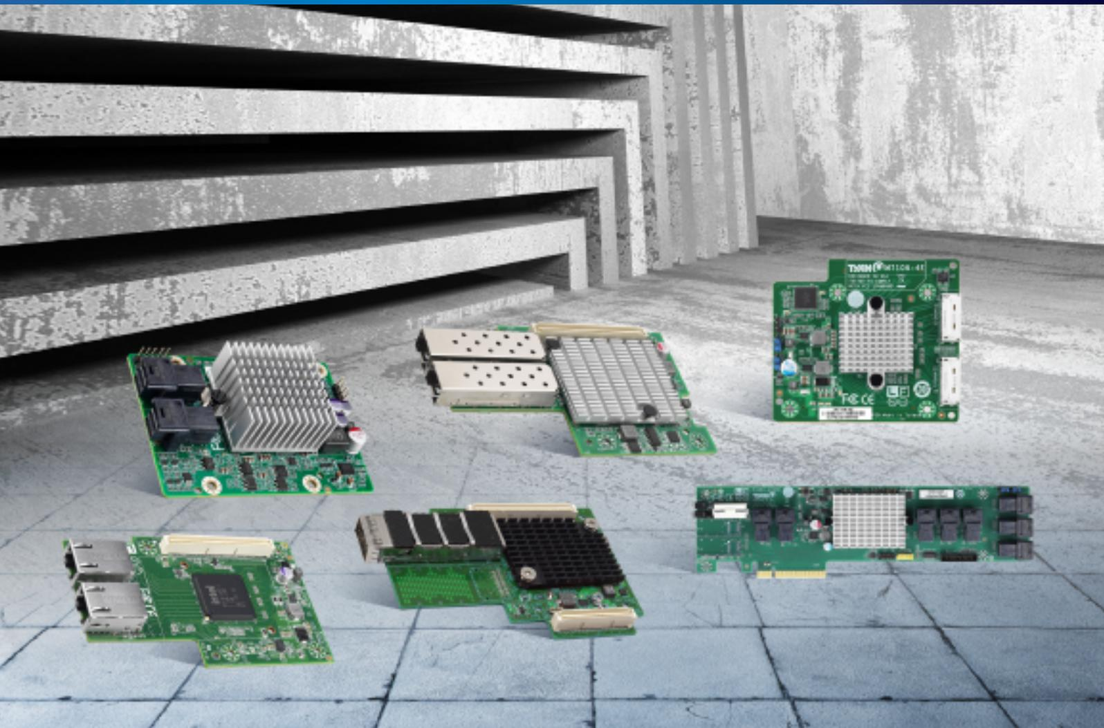
**T**YAN adopts a modular I/O approach with many of its server platforms. This design flexibility allows customers to deploy a single base motherboard with a wide variety of networking and storage options. It also allows customers to upgrade portions of their server without having to replace core parts such as the motherboard.
