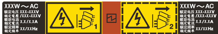
Figure 38. Hot-swap power supply label on the cover
