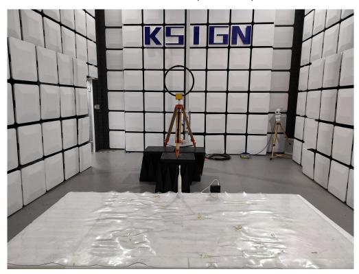
Radiated Measurement (Above 30MHz)
