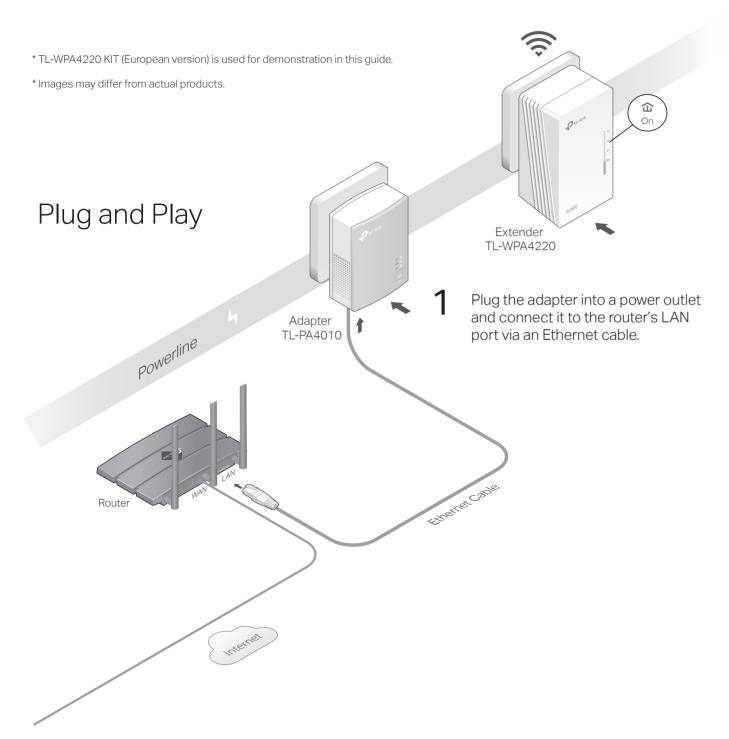
Plug the extender into a power outlet on the same electrical circuit.
