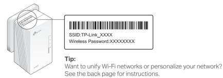
**Note:** If you cannot find the default SSID in your Wi-Fi network list, this means that the extender has been connected to a OneMesh router and automatically copied its Wi-Fi settings. For more information, see **OneMesh<sup>TM</sup> with Seamless Roaming** on the back page.
