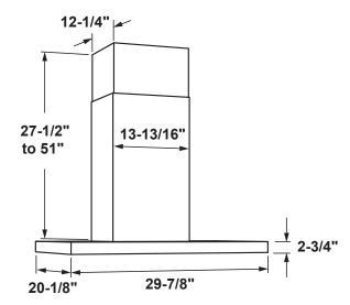
30"models require a 30"-wide opening \*The supplied duct cover fits 7'-7" to 10'-6" ceiling heights (12' ceiling height with optional high celling kit UX12DC9SLSS/UX12DCBLTS) (14' ceiling height with optional high celling kit UX14DC9SLSS/UX14DC9BLTS)
