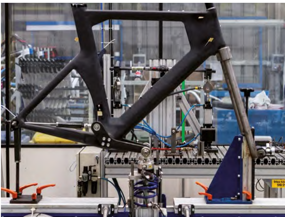
The global stiffness test is used by manufacturers to measure frame deflection. The rear dropout is fixed in place and a force applied to the side of the headtube flexes the entire frame. The amount of movement at the headtube for a given force is recorded in millimeters.
