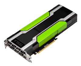
The NVIDIA Tesla P4O is purpose-built to deliver maximum throughput for deep learning deployment. With 47 TOPS (Tera-Operations Per Second) of inference performance and INT8 operations per GPU, a single server with 8 Tesla P4Os delivers the performance of over 140 CPU servers.
