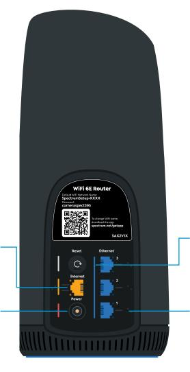
Internet (WAN) port - Connect - network cable to the modem for wide area network connection.
