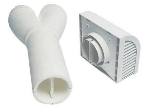
**FV-WC04VE1** WhisperComforts FV-WC04VE1 polypropylene wall cap accessory with Styrofoam adaptor conveniently allows both exhaust (from the right) and supply (from the left) airflow through a single 5.5"-5.75" penetration in the building envelope. Due to the dividers inside of the unique Y-shape chamber and the new wall cap, cross contamination is prevented.
