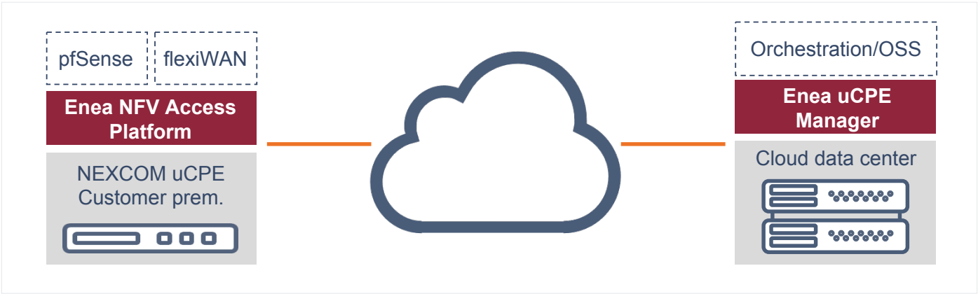
Figure 3. Block diagram of demonstration setup including Enea NFV Access Platform as the provider of all network functions virtualization infrastructure (NFVI)
