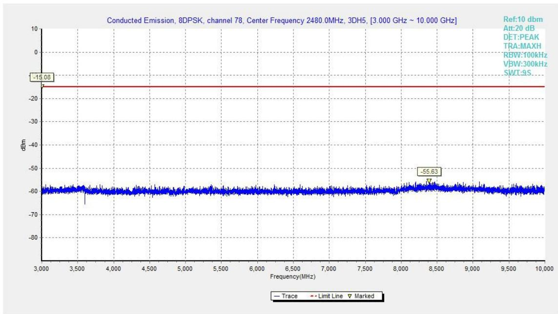
Fig.62. Conducted spurious emission: 8DPSK, Channel 78, 3GHz - 10GHz
