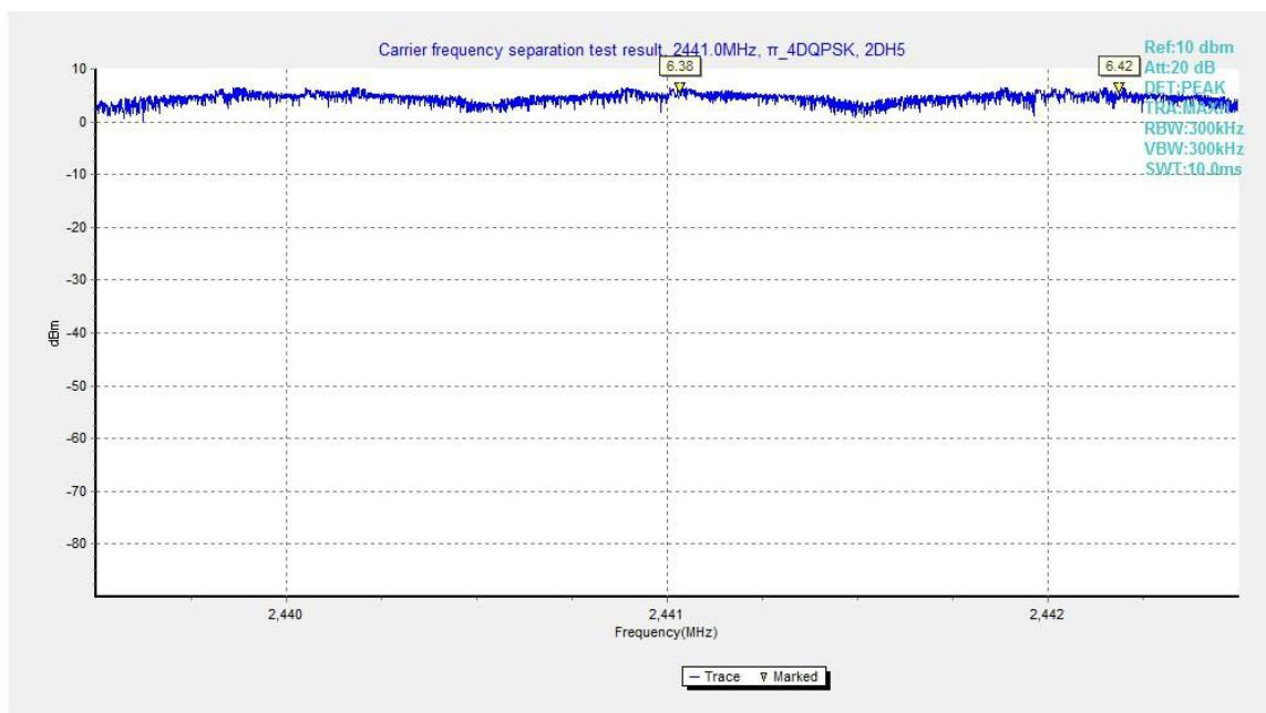
Fig.92. Carrier frequency separation measurement: π/4 DQPSK, Channel 39
