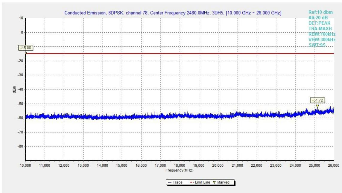
Fig.63. Conducted spurious emission: 8DPSK, Channel 78, 10GHz - 26GHz
