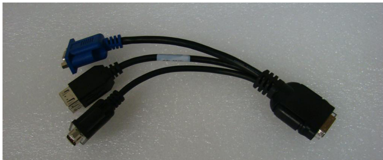
Figure 1-5. Adapter to Provide USB, COM, and VGA Ports
