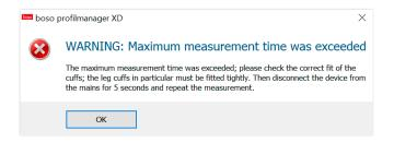
This message appears after an excessively long measurement time; the maximum duration allowed is 150 seconds.
