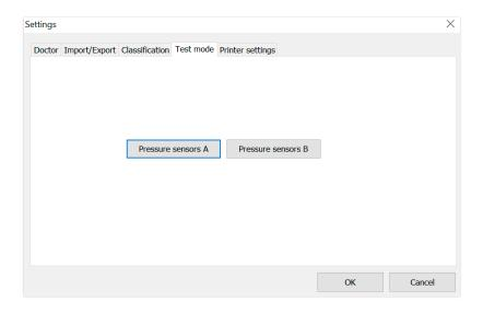
The test mode is activated using the "Pressure sensors A" and "Pressure sensors B" button. Clicking on the "Finish test" button ends test mode.
