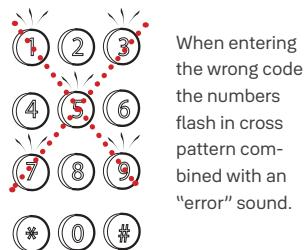
When entering the wrong code the numbers flash in cross pattern com-bined with an "error" sound.
