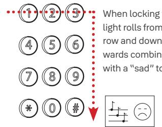
When locking the light rolls from top row and down-wards combined with a "sad" tone.
