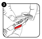
4. Gently pull the audio-lines from the cartridge, taking care to pull from the terminal connector and not the wire itself.
