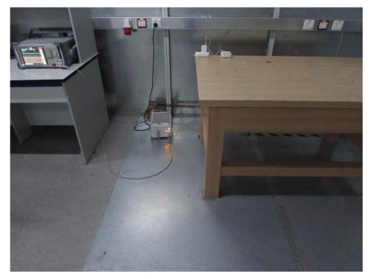
Radiated Emission From 9kHz to 30MHz
