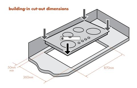
Note: If a barrier is not required, a minimum gap of 30mm is needed under the cooktop.
