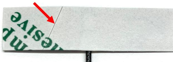
1. Find cut line on flex back side
