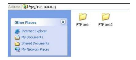
You can also access the FTP server by external network. Please type in address ftp://WAN IP to access to it.
