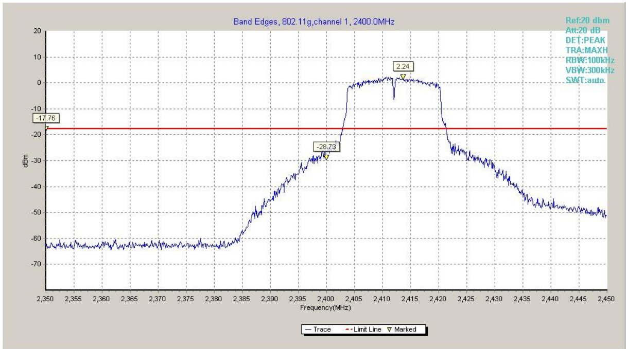
Fig.A.5.3 Band Edges (802.11g, Ch 1)
