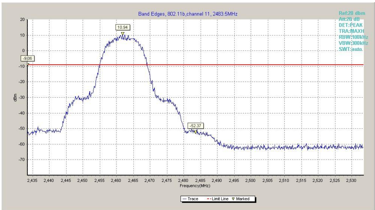
Fig.A.5.2 Band Edges (802.11b, Ch 11)
