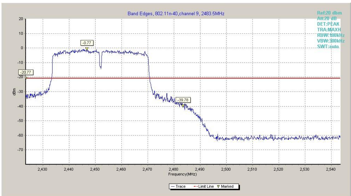
Fig.A.5.8 Band Edges (802.11n-HT40, Ch 9)
