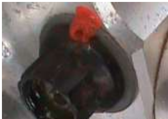
Figure 13 - Torque seal installed
