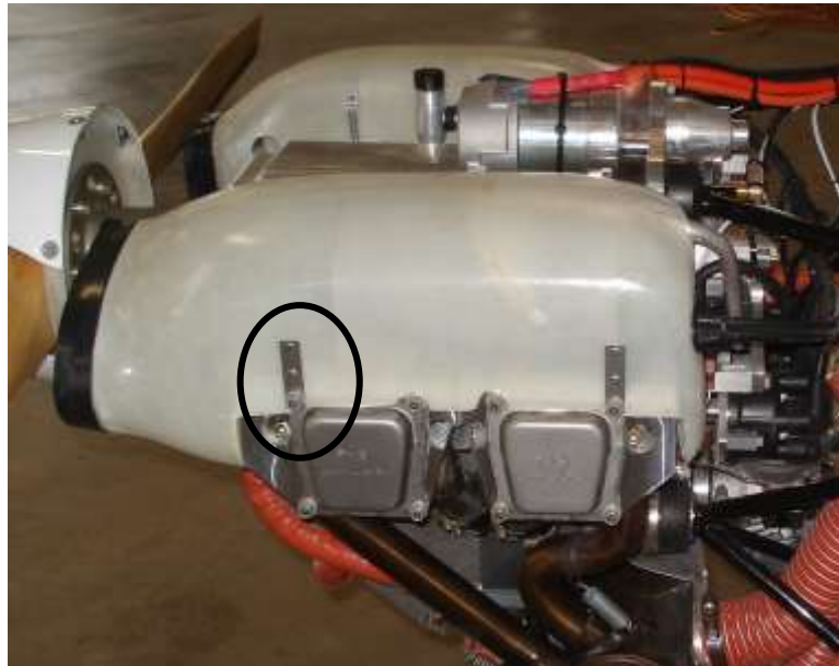
Figure 32 – Air Duct Hard Point Reinforcement
