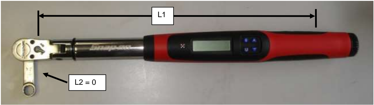
Figure 30 – Torque Wrench & Crowsfoot Adaptor Setting 2
