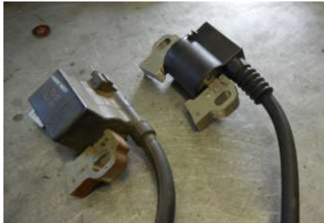
Figure 44 – Different Ignition Coil Models (Honda on Left, Jabiru on Right).
