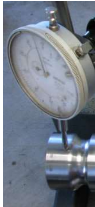
Figure 48 – Dial Indicator Position for Crankshaft & Prop Flange Run Out
