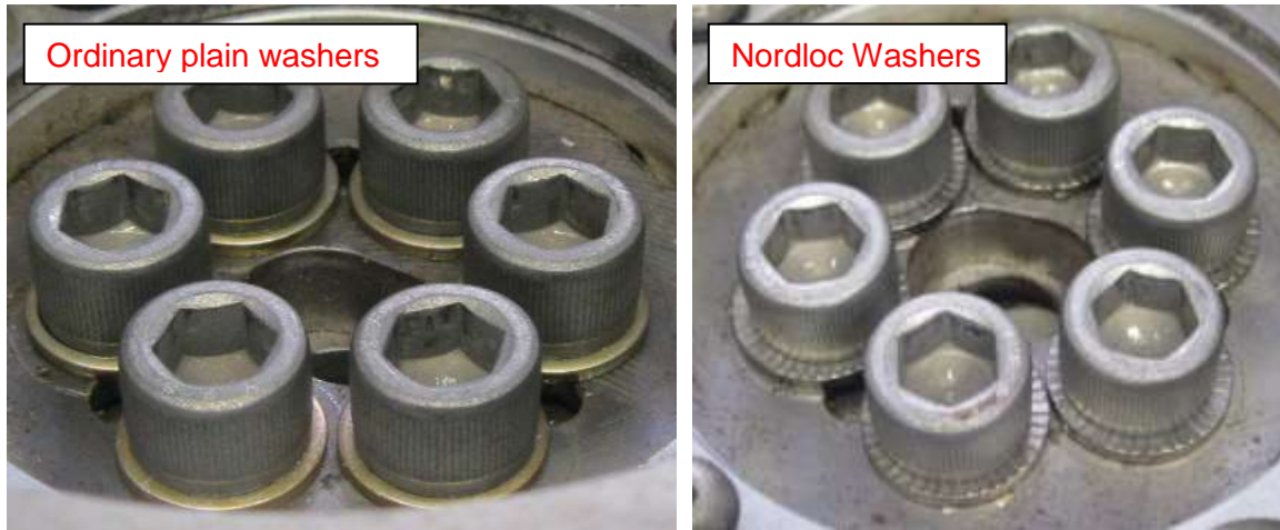
Figure 45 - Plain washers compared to Nordloc washers
