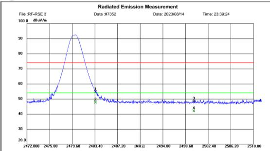
Site LAB Chamber 2 Limit: FCC Part15C
