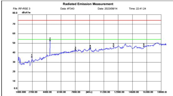
Site LAB Chamber 2 Limit:FCC Part15C
