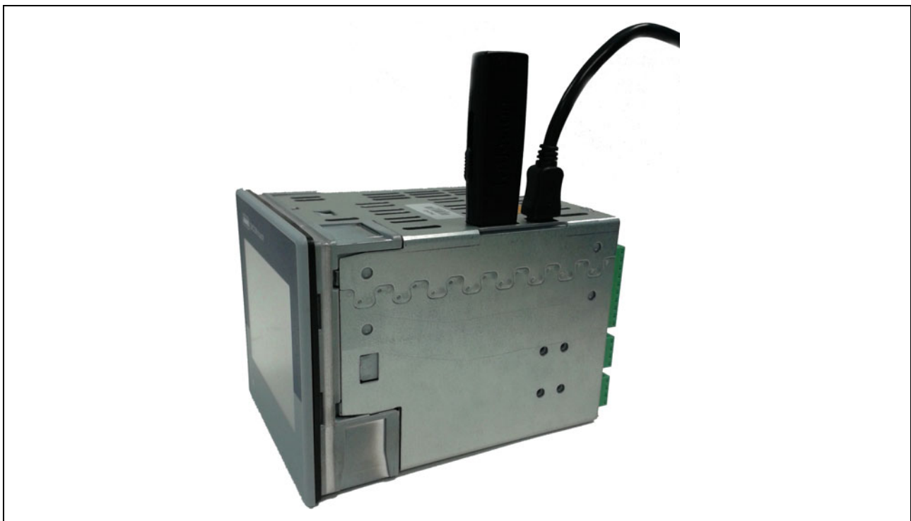
Figure 107: JUMO DICON touch with USB device and USB host interface
