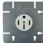
45126 Flush Mount Range Receptacle, 3 pole, 4 wire, grounding 50A/120-240V Nema 14-50R
