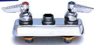
B-1100-LN 3-1/2" B-1110-LN 4" T&S Workboard Faucet, deck mounted, bronze body, removable seats, 6-1/2" x 2" wide chrome plated escutcheon, 4" centers, 1-1/2" long shanks & 1/2" IPS thread, spout separate
