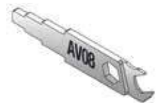
AV08 Spartan cartridge, packing and union tool. Will remove 1/2", 3/4", 1" and 1-1/4" sizes. Can also be used to keep the EB type cartridges in place when removing actuator.
