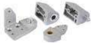
11-1545L Left Hand 11-1545R Right Hand Amarlite Door Pivots for commercial doors. Aluminium Finish, Bronze available Includes Top And Bottom Door Portions And Top And Bottom Frame Portions 3/4" offset pivots for aluminium doors and frames For flush door / frame and 1/8" recessed door applications Weather resistant
