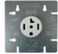
45125 Flush mount Dryer Receptacle, 3 pole, 4 wire grounding 30A/120- 240V Nema 14-30R
