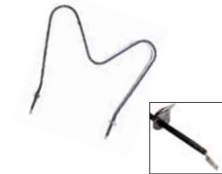
316075104 (1950/2600W/240V) Frigidaire Range bake element. 19.50"W x 18.50"L x 3.50" insert
