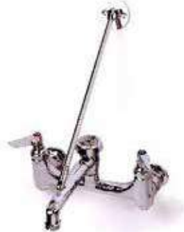
B-0665-BSTR T&S Service sink faucet, built-in screwdriver stops, 8" centers, 2-3/8" clearance from the wall to center of faucet, polished chrome plated finish, vacuum breaker with 3/4" garden hose thread and pail hook and top support wall brace.
