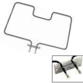
UB813 (2500W/240V) Frigidaire Range bake element. 20.25"W x 14.5"L x 1.88" insert
