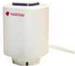
ME1607 Normally Open (Stem Up) ME1707 Normally Closed (Stem Down) Spartan Compact Thermolectric Spring Return Actuator. 24V Direct Acting. Highly refined wax filled element with piston/stem and patented packless elastomer seal. Silent, extremely compact, inherently fail safe and can operate on hot and cold water, and low pressure steam to 15PSI.
