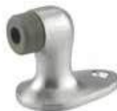
J4573 Chrome Floor Door Stop with rubber bumper. 2"H, Solid brass construction. Threads in then has extra screw to hold in place. Meets ANSI
