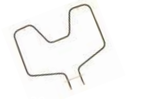
WS01F02247 (2585W/240V) G.E. Range bake element. 18-1/8" W X 15-3/4" L X 2-3/8" insert
