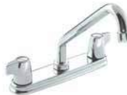
77924 Chrome Moen II Series, two handle kitchen faucet, small lever handles, washerless, Quick Connect
