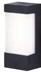
LED Outdoor Fixture 7W, 500 Lumens, 3000K, 30000hrs, Acrylic lens, plastic body 4-1/4"W X 9-1/2"H X 3-1/4"D BRWL-SQ6W-N-BK
