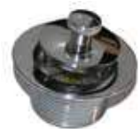
343CP-S 1-5/8" X 16TPI 343CP-L 1-7/8" X 11.5TPI OS&B lift and turn drain assemblies, please note size of strainer and threads per inch, chrome top, tub drain stopper
