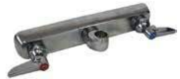
B-1125-LN 8" Splash Back Mounted, Bronze body, removable seats, 10-1/2" long X 2" wide chrome plated escutcheon, 8" centers, 1-1/2" long shanks, 1/2" IPS thread
