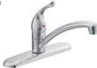
67425 no spray 67434 w/side spray Moen "Chateau" chrome single lever kitchen faucet, washerless, 3 hole 8" install, c/w flexible 3/8" supply connections and 9-1/8" spout
