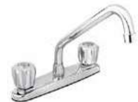
3065 Chrome Belanger 8" swivel spout, 8" centers, 1/2" IPS connections, Brass waterways and ceramic cartridge
