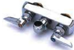
B-1115-LN 4" T&S Splash back mounted, bronze body, removable seats, 4" centers, 6-1/2" x 2" wide chrome plated escutcheon, 1-1/2" long shanks and 1/2" IPS thread, spout separate
