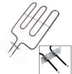
318255605 (2750W/240V) Frigidaire Range Broil Element. 12"W x 19.5"L x 3.5" insert
