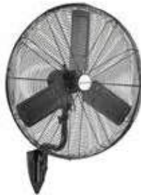
WMKD24-3SP 24" Stationary WMKD24-OSC 24" Oscillating Canarm Commercial Circ Fan. Creates a gentle air movement. 3 Speed thermally protected motor, industrial grade aluminum blades, OSHA guard, c/w 10' 120V grounded cord, wall mounting hardware. 30" also available.
