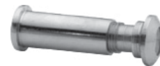
25-D4841B Brass 25-D4841N Nickel Door Viewer 160° Angle Of Vision, 15/32" Bore Size, Adj. 1-3/8" to 2-1/8" plastic lens
