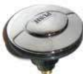
330BCP-S 1/4" Post 330BCP-L 5/16" Post OS&B Clicker cartridge, brass top chrome plated, used in tubs and lavs, note post sizes
