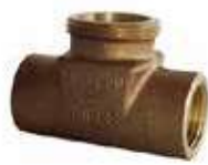
V243-12N 1/2" Female Inlet and Outlet Spartan 2-Way Zone Control Valve Body. Use EB, EP or EV series cartridges sold separately. For hot and chilled water and 50% glycol. Compatible with complete line of Spartan control valve actuators.
