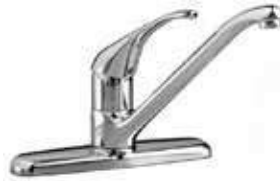
4205000.002 Chrome AmStd Reliant kitchen faucet. Ceramic disc valve, 8" install, cast brass construction, metal handle, higher longer spout, 1/2" male thread inlets
