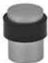
25-4613SS Architectural door stop. Stainless steel type 304, black rubber bumper. 1-9/16"H x 1-11/16"Dia. Screw included.
