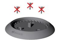
The sensor base must be fixed to the ground (substrate such as concrete, asphalt) with a two-component adhesive from a leading supplier (e.g., DELO®, 3M®, ...).
