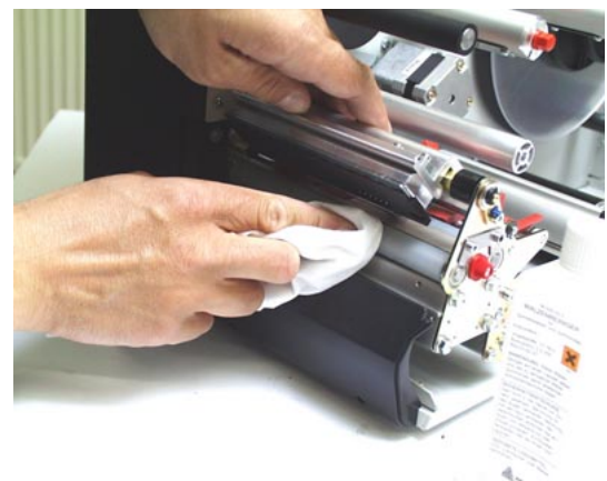
Fig. 4 Rotate the printhead upwards before cleaning it.
