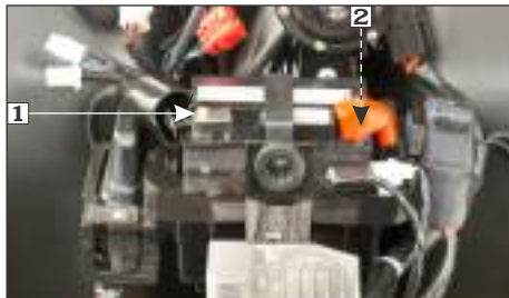
(1) (-)ve terminal (2) (+)ve terminal
