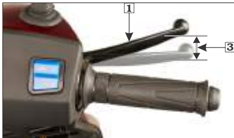
(1) Front brake lever (3) Free play: 10-20 mm
