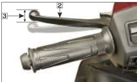
(2) Integrated brake lever (3) Free play: 10-20 mm
