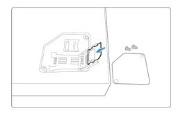
4. After loading the SIM card, push the buckle left to lock the SIM card slot tightly.
