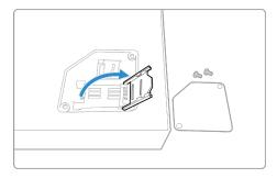
3. Look for the location of the SIM card gap and insert the SIM card. Activated Nano SIM card can be adapted to Standard size to fit into SIM card gap
