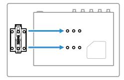
8. Hook the lower edge of the DIN rail under the buckle.
