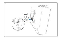
9. Pull the device up and let the hook above the buckle hook the upper edge of the DIN rail. Use a pair of slotted TS35 DIN rails (35mm high x 7.5mm deep) cut to slightly longer than the length of the assembled system, and attach to a strong wall or other rigid surface using low-profile screws.
