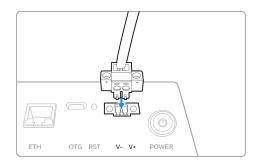
12. Lock the screws tightly to avoid loosening.
