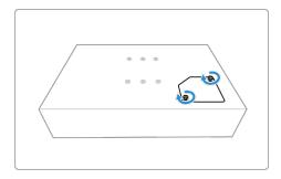
6. Remove the 6 countersunk head screws.
