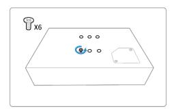
7. Replace with countersunk head screws to fix the DIN buckle. Be mindful of the direction. Do not overtighten.
