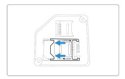
5. Put on the SIM cover and tighten the two screws (pay attention to the front and back of the cover plate)
