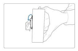
10. Install the antenna and fix it on the connector.
