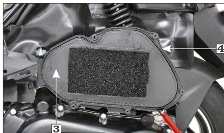
(3) Air cleaner element holder component
