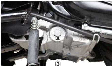
(3) Oil strainer screen cap
