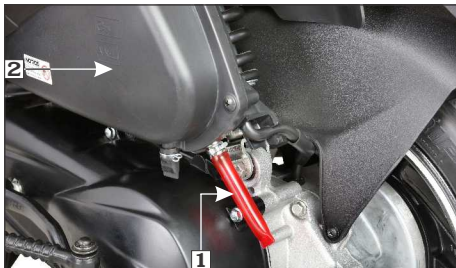
(1) Drain tube (2) Air cleaner assembly
