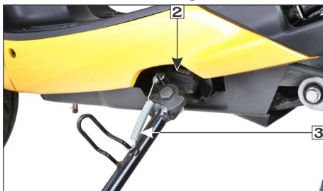
(2) Side stand switch (3) Side stand spring
