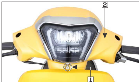
(1) Screw (2) Handlebar cover
