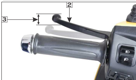
(2) Integrated brake lever (3) Free play: 10-20 mm
