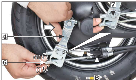
(6) Second adjuster nut (7) Joint (i) Decrease free play (ii) Increase free play
