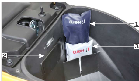
(1) Tool kit (2) Center compartment (3) First aid kit
