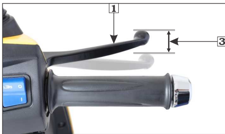
(1) Front brake lever (3) Free play : 10-20 mm
