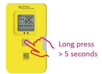
The following information will be displayed on the screen. While the information "\*\*\*START\*\*\*" will be displayed **as a ticker**, keep pressed the multifunctional button and hold the multifunctional button for at least 5 seconds.
