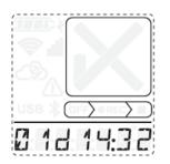
By a short press to the multifunctional button, the information *SCHEDULED START* will show as ticker on the display with above information about the time till the device will start recording.
