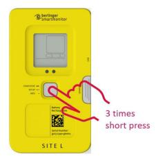
The display starts showing after press quickly 3 times following screen
