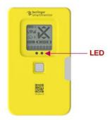
If no start delay is configured, the device goes directly into the Record modus and shows **REC** on the display as confirmation that the device is recording.
