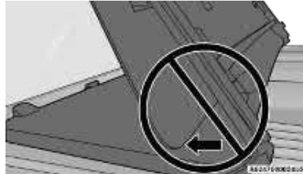
Incorrect Folding – Will Cause Damage
