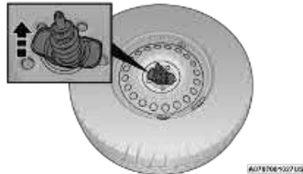
Reinstalling The Retainer
