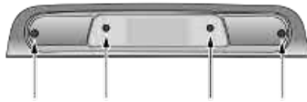
CHMSL Mounting Screw Locations
