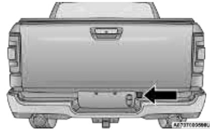
Access Hole Cover Location
