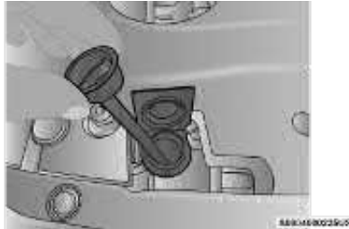
Coolant Reservoir Dipstick
