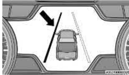
Lane Approached (Flashing Yellow Lane Line) With Flashing Yellow Telltale
