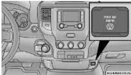
Center Stack Power Inverter
