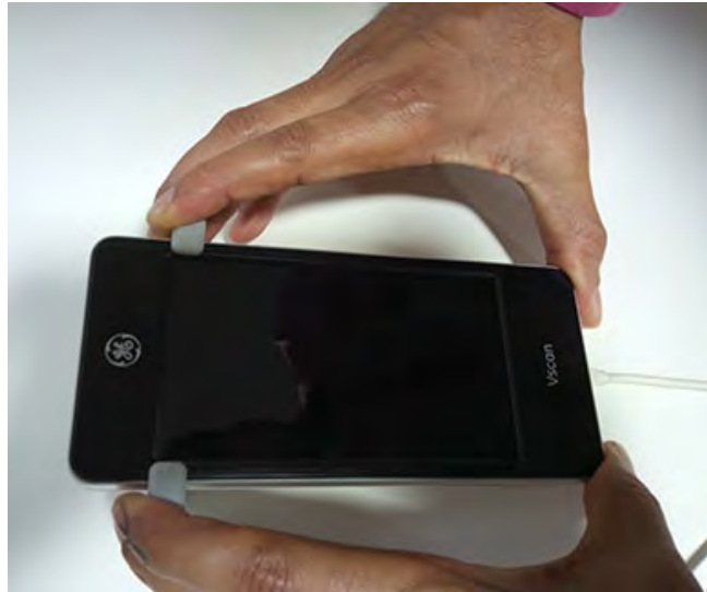
Figure 3-8. Slide stand on device
