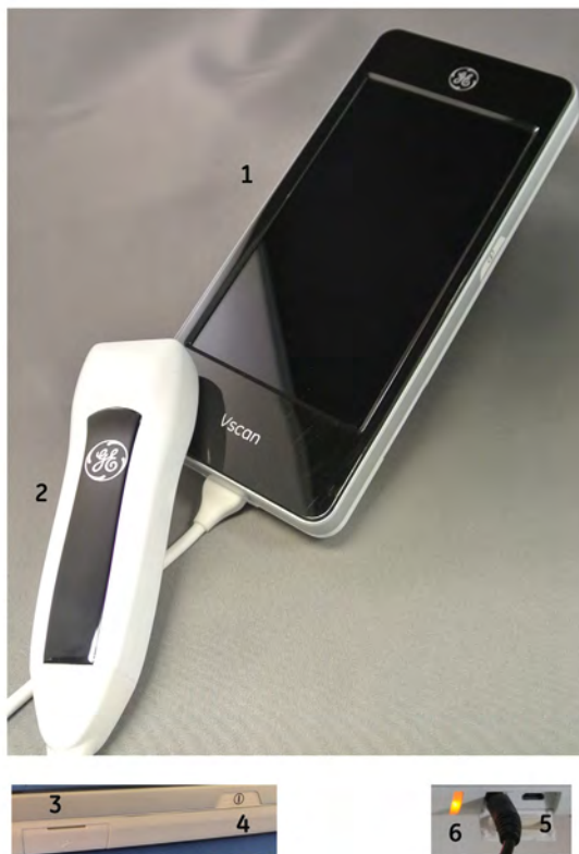
Figure 3-2. Vscan Extend with a Sector probe
