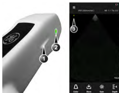
Figure 5-2. Dual probe: Orientation mark, phased array active
