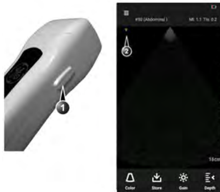
Figure 5-1. Sector probe orientation
