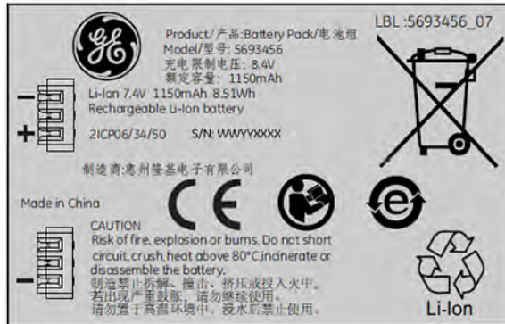
Figure 2-3. Vscan Extend battery label
