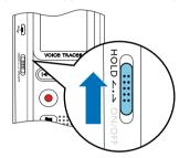
Slide the HOLD switch down to the Off position to disengage the HOLD.
